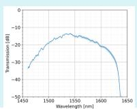
When the optical input power of the DUT is set to 0 dBm, the transmission already represents the IL and does not require any further analysis. To know the set-up losses, a reference measurement without the DUT can be conducted. If one measures an imbalanced MZM, the spectra will show an interference pattern.
