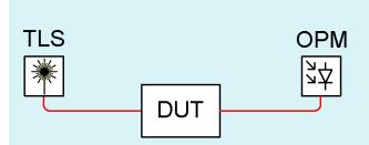
DUT: OPM: TLS: Device Under Test Optical Power Meter Tunable Laser Source
