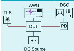
AWG: Arbitrary Waveform Generator DSO: Digital Storage Oscilloscope
